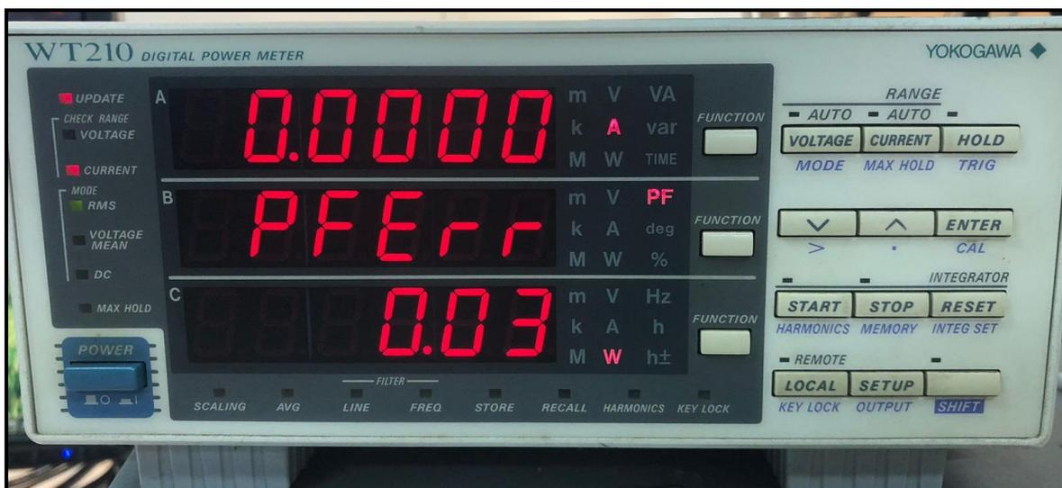
**Figura 22- Wattímetro Digital Yokogawa WT-210.**
