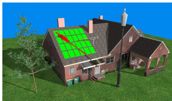
(d) Shadow evaluation on the photovoltaic array installed on the roof of the house [40].
